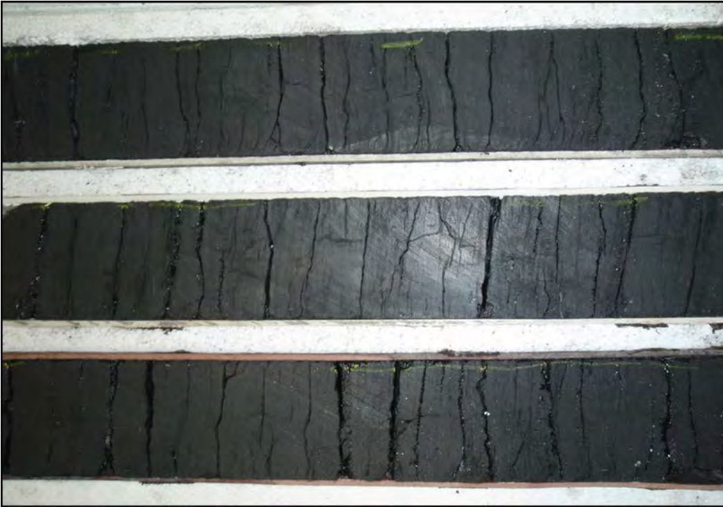
Figure 20 Core photo of Bindah 3 core showing macro-scale appearance that is characteristic of Cooper Basin deep coals
