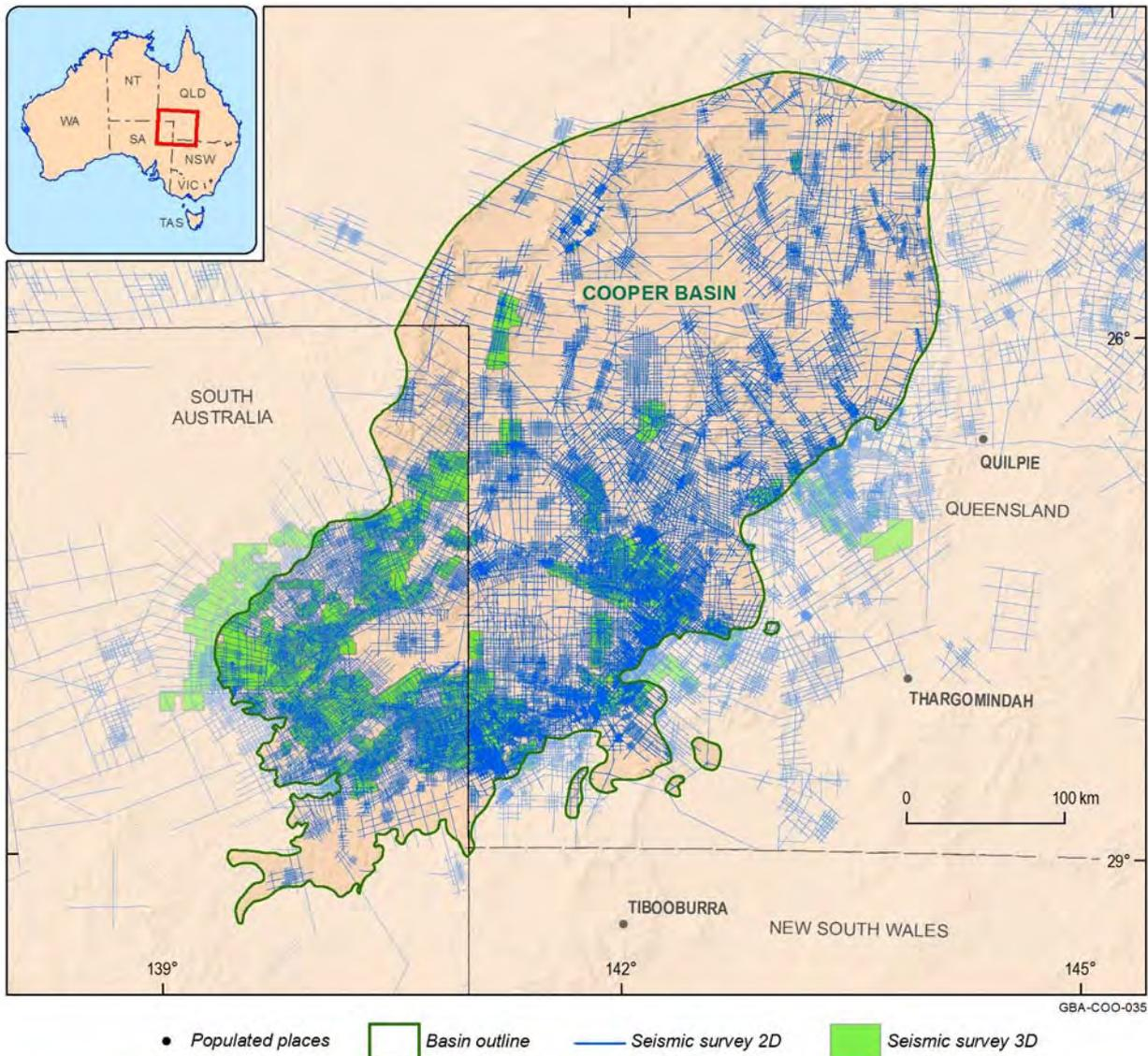
**Figure 9 Cooper Basin seismic data coverage (two-dimensional and three-dimensional)**
