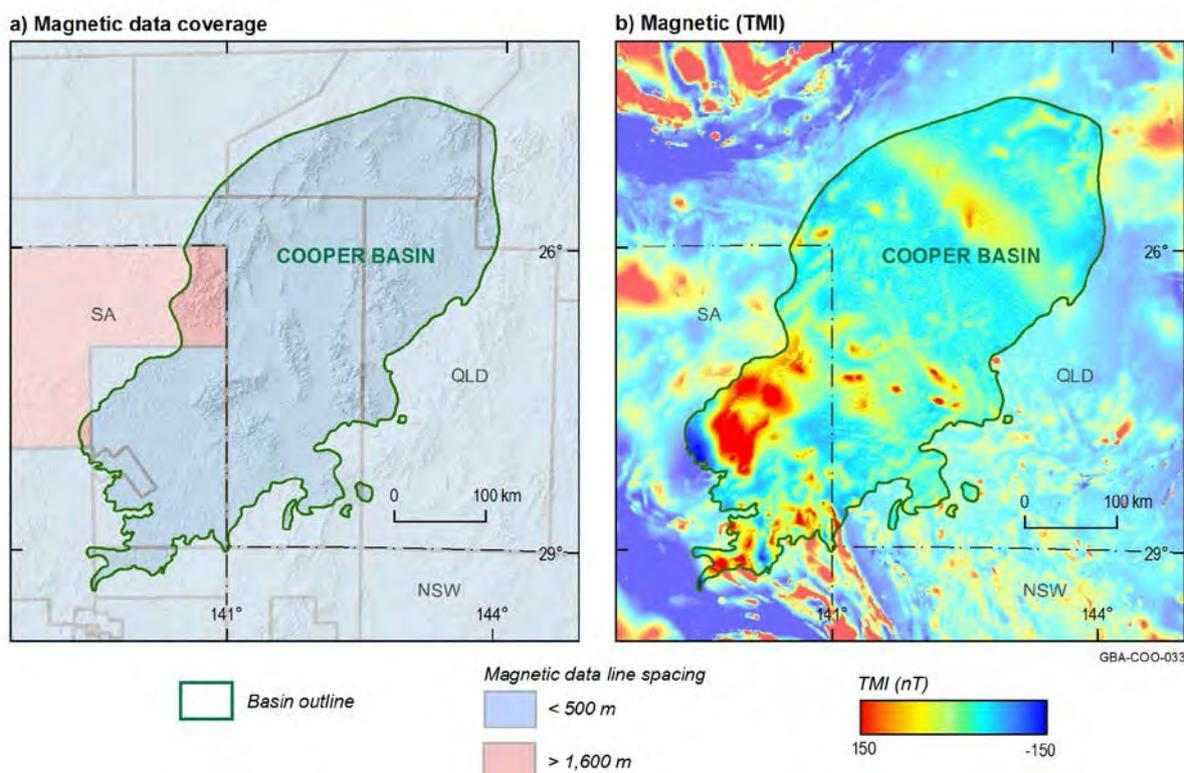
**Figure 11 a) Distribution of magnetic survey by resolution; b) Regional TMI (Total Magnetic Intensity) data coverage**
