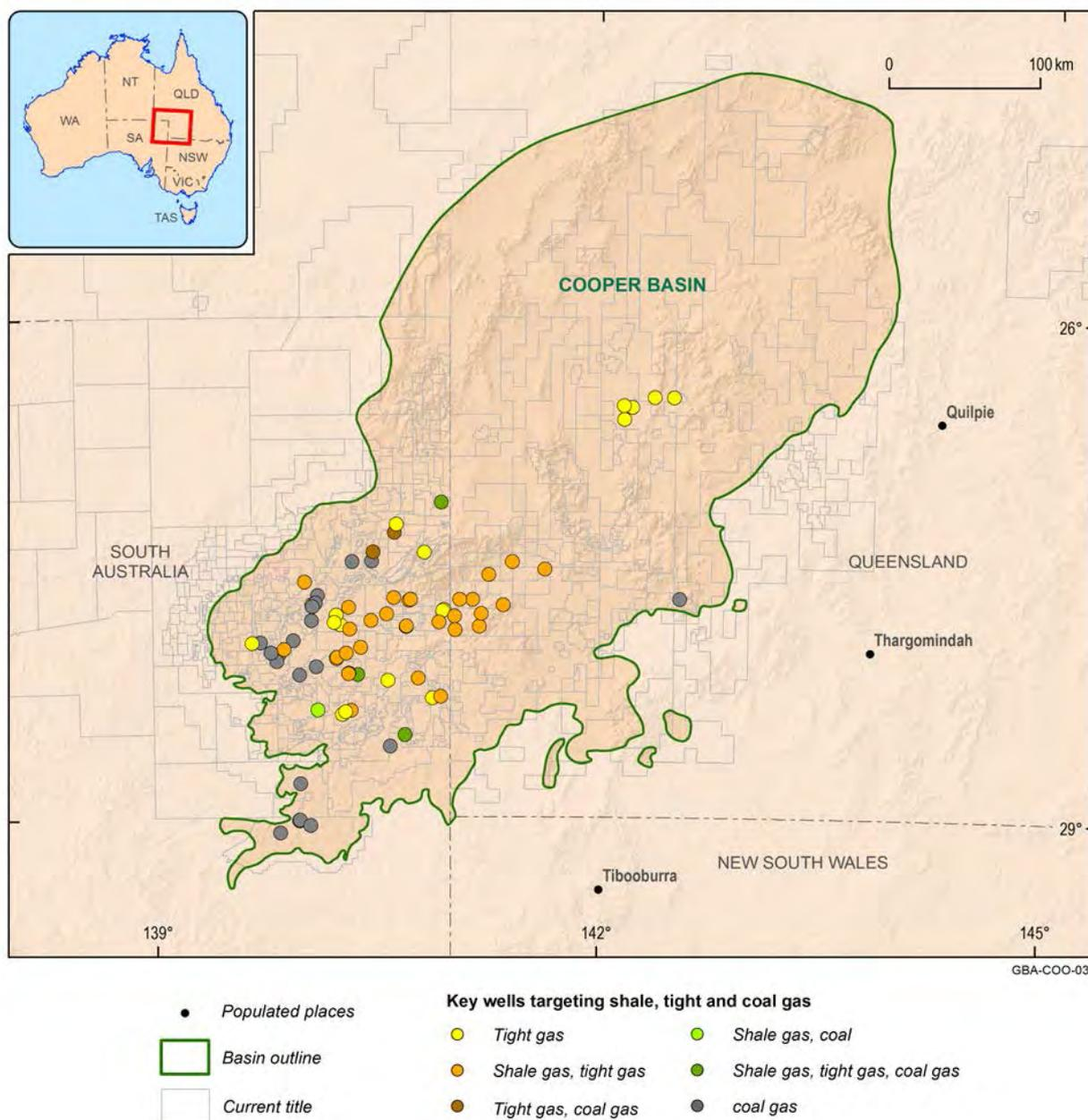
**Figure 8 Distribution of key wells used to characterise reservoirs for the shale, tight and deep coal gas plays assessed in this study**
