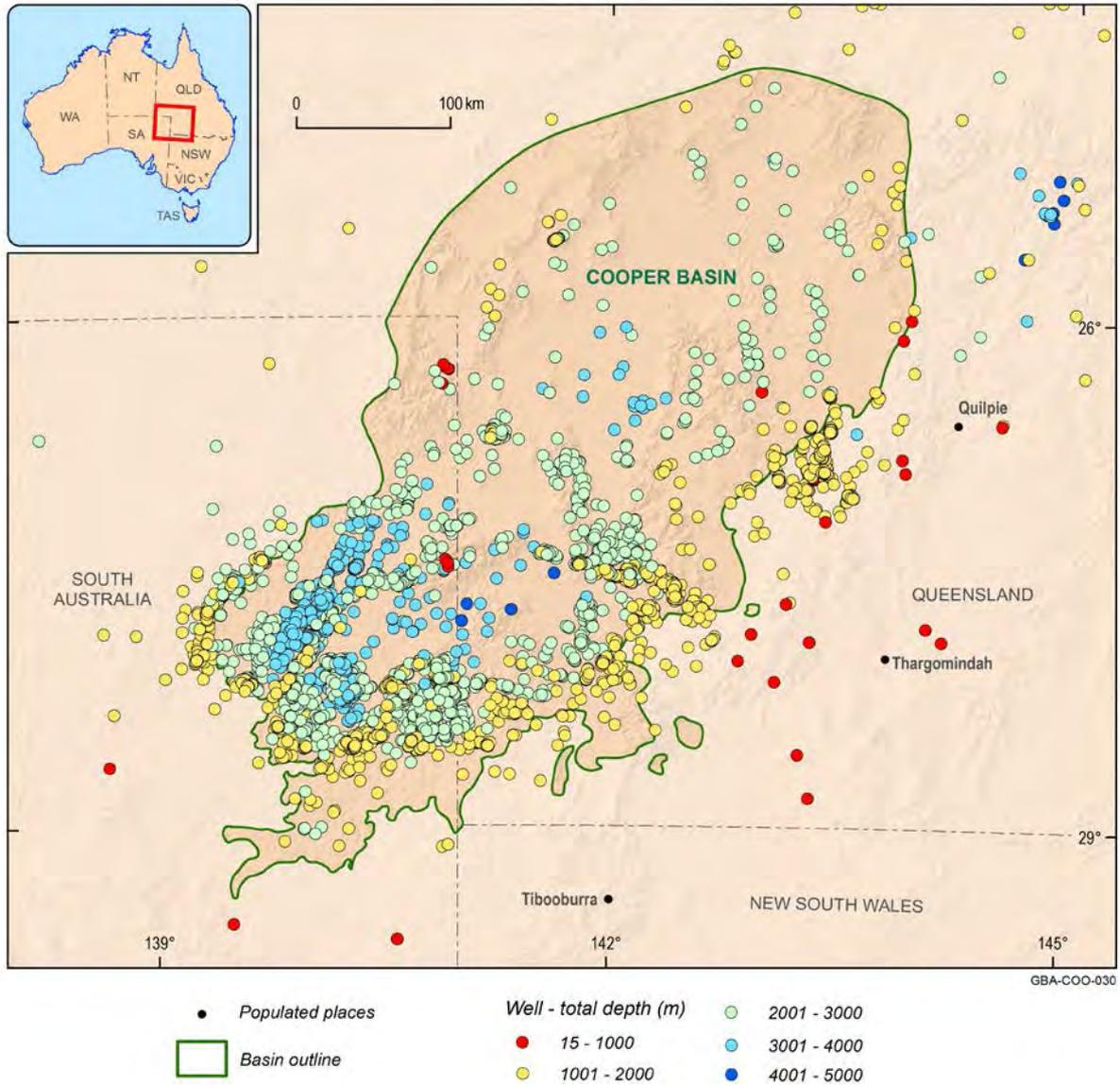
**Figure 7 Distribution of wells and bores in the Cooper GBA region, classified according to their depth of penetration**
