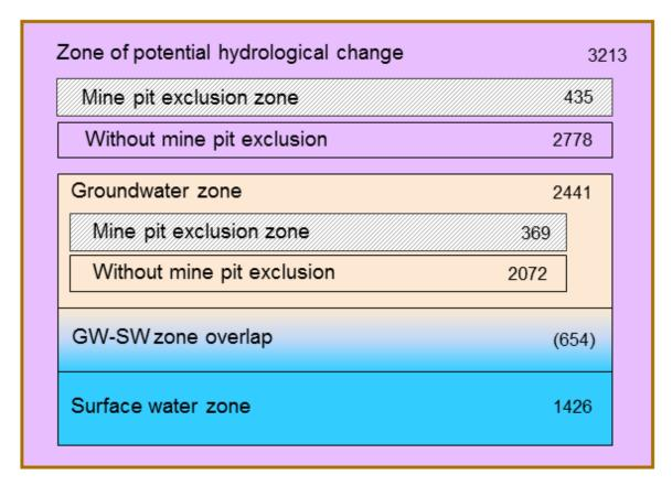
Figure 18 Summary of the areas (km<sup>2</sup>) of the zone of potential hydrological change and its surface water and groundwater components for the Hunter subregion
