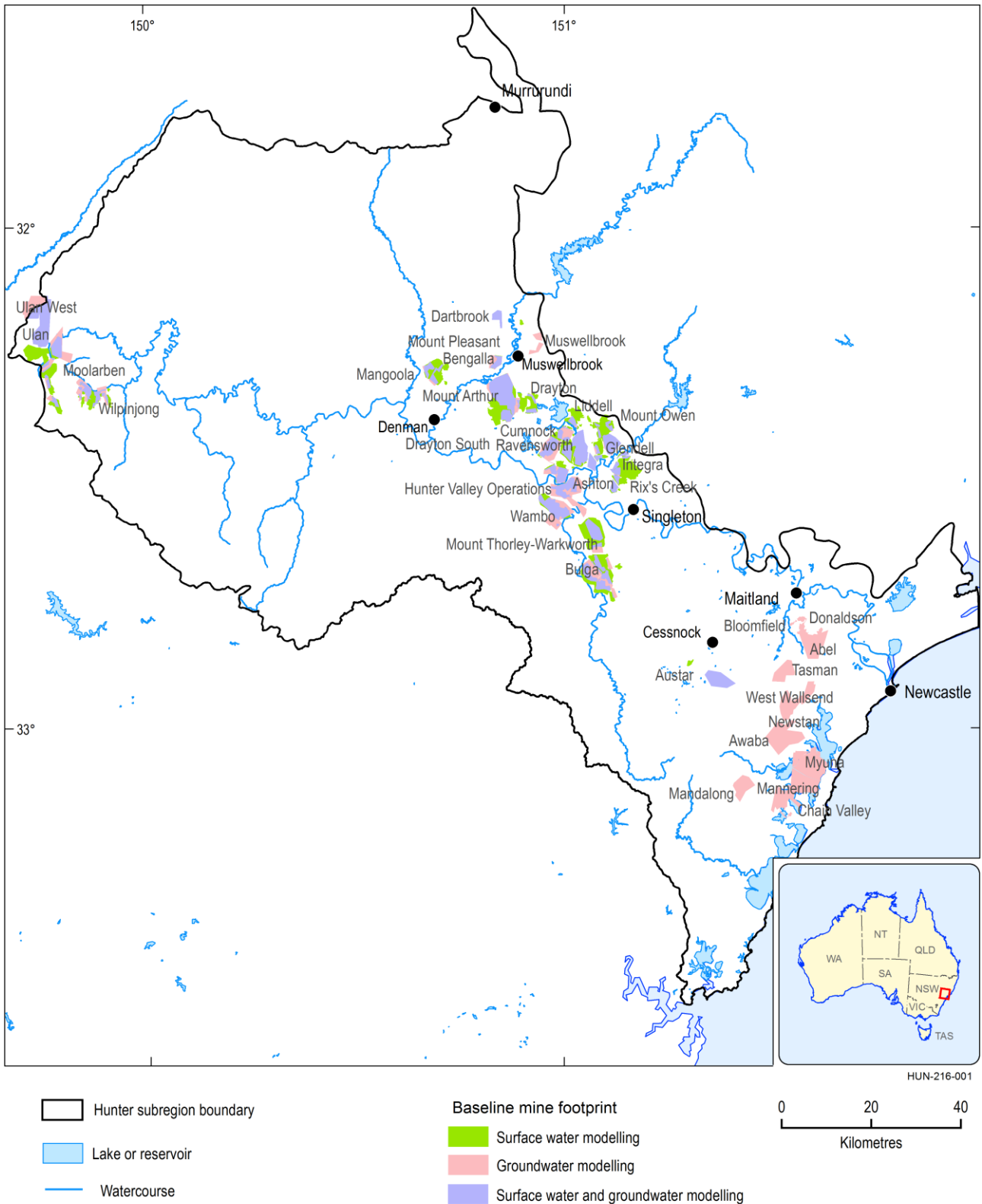
Figure 38 Maximum footprint areas for baseline mines used in surface water and groundwater models
